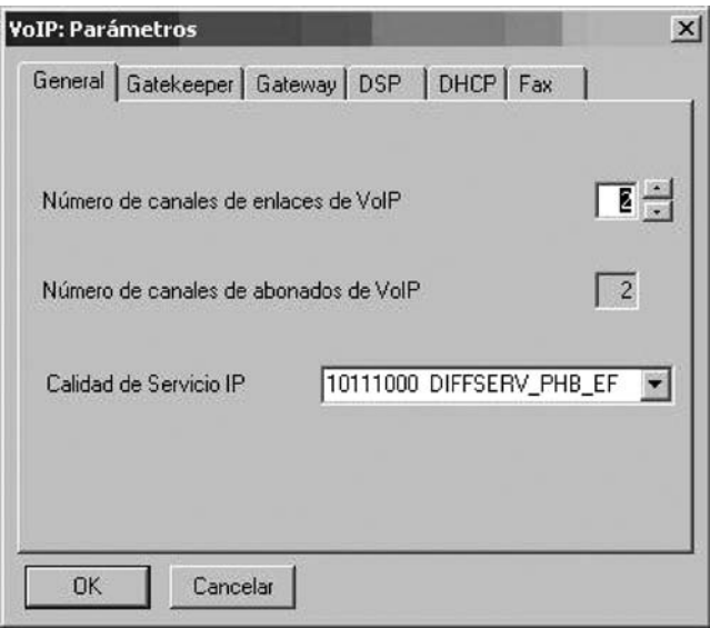
Figure 4.17 DiffServ configuration in an IP-PBX.
