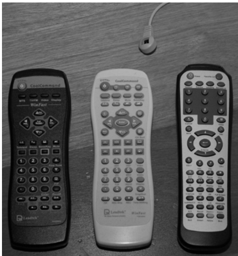
Figure 3-1. Three remote controls shipped with TV capture cards and an IR sensor
