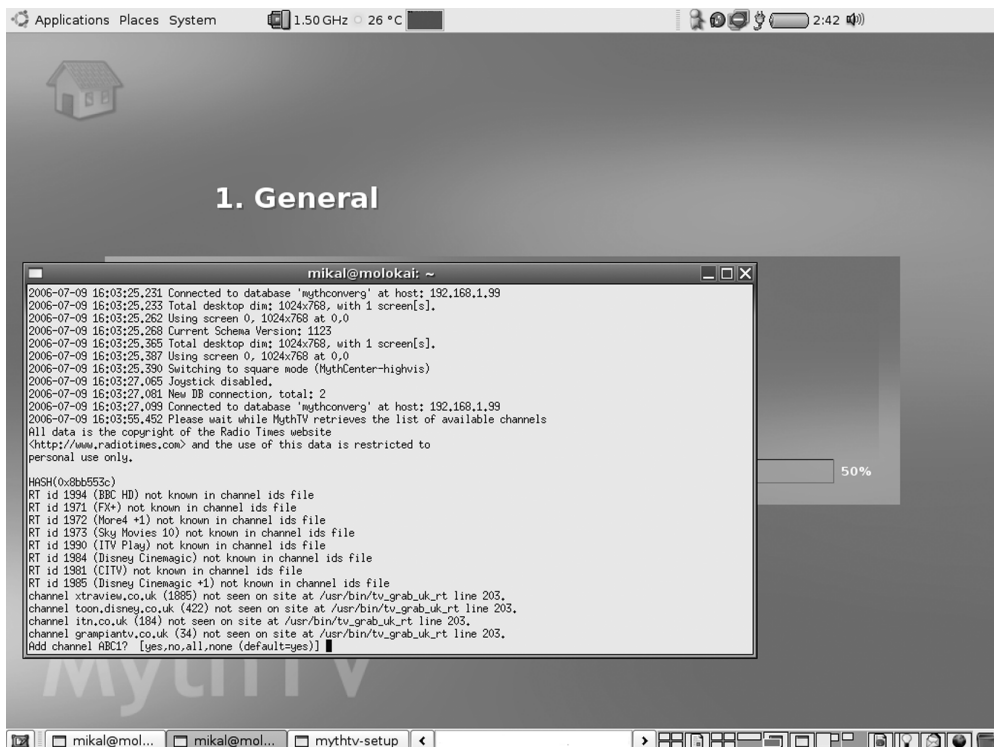
Figure 4-13. The XMLTV grabber is configured in the terminal.
