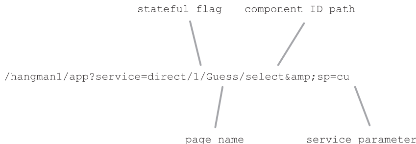
Figure 7.9 The direct service URL identifies the page and component and allows for application-specific service parameters.
