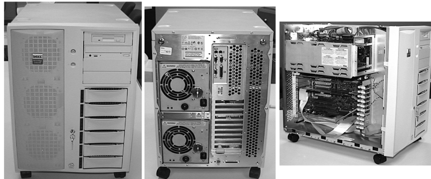
Figure 6-50 Server with hot-swappable, redundant power supplies.
