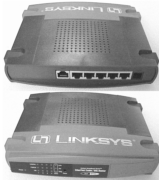
Figure 6-25 DSL/cable modem router and four-port Ethernet switch.
