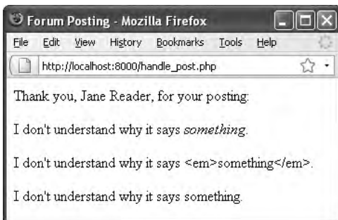
Figure 5.10 The resulting PHP page shows the original post as it would look if printed without modification, the effect of htmlentities(), and the effect of strip_tags().
