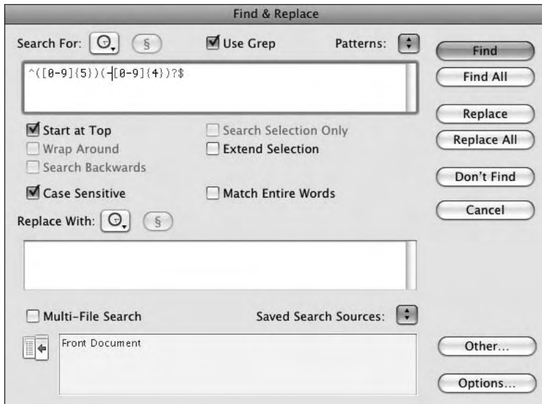
Figure 13.1 Within BBEdit's standard Find & Replace dialog box, you have the option of using regular expressions (even across several files or folders) by checking the Use Grep box. BBEdit can also store regular expression patterns for you and has some built in.
