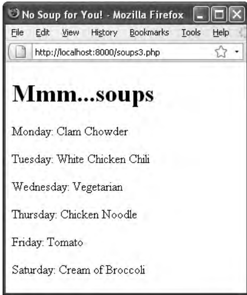
Figure 7.4 The execution of the loop for every element in the array generates this page. The foreach construct allows the script to access each key and value without prior knowledge of what they were.
