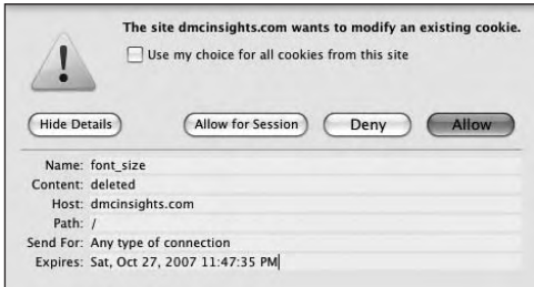
Figure 9.14 When the setcookie() function is used with a name but no value, the existing cookie of that name is deleted. The expiration date in the past also guarantees proper destruction of the existing cookie.
