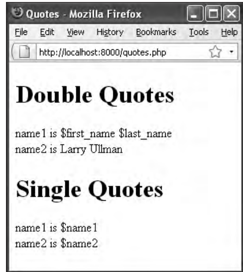
Figure 2.7 The different quotation marks (single versus double) dictate whether the variable's name or value is printed.
