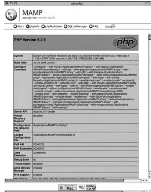
Figure A.22 The phpinfo() function prints the location of the active php.ini file as well as all the configuration information.
