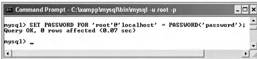
Figure A.17 You should establish a secure root user's password immediately after you install the software.
