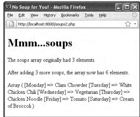
Figure 7.3 A direct way to ensure that the new elements were successfully added to the array is to count the number of elements before and after you make the additions.
