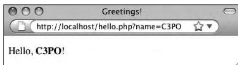
Figure 3.18 Any value assigned to name (lowercase) in the URL is greeted by the PHP script.
