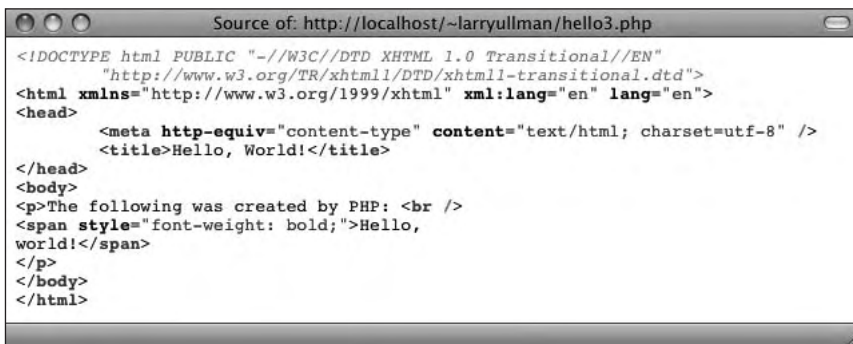
Figure 1.12 The \n in the print statement separates the Hello, world! line from the other HTML tags (note the placement of the closing paragraph tag here and in Figure 1.10).
