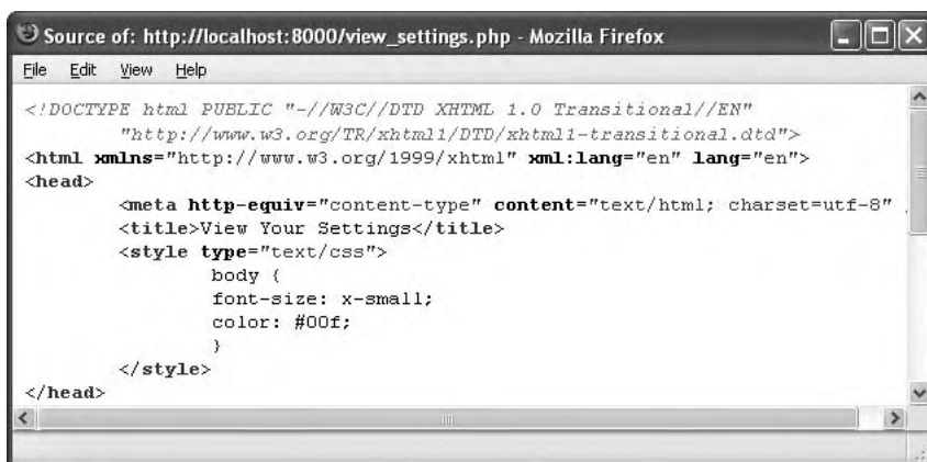
Figure 9.10 By viewing the source code of the page, you can also track how the CSS values change.
