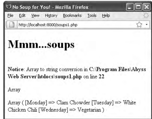
Figure 7.1 Because an array is structured differently than other variable types, a request to print an array results in the word Array (and an error, depending upon the version of PHP and its settings). On the other hand, the print_r() function prints the array's contents and structure.
