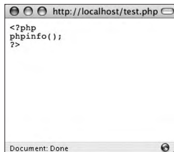
Figure 1.7 If you see the raw PHP or HTML code, then either PHP isn't installed correctly or the extension you used ( .php ) isn't treated as a PHP file by the server.
