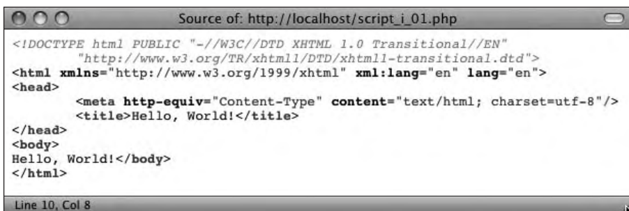
Figure i.10 By viewing the source code received by the Web browser, you can see the HTML created by PHP and sent by the server.
