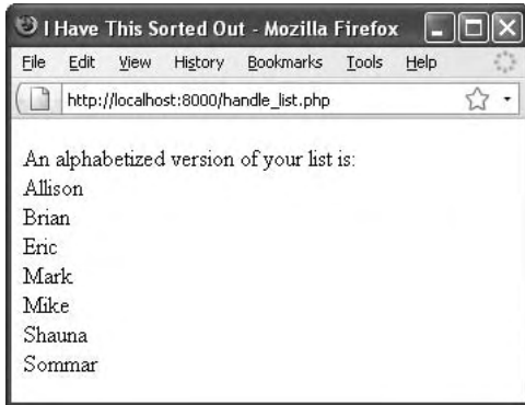
Figure 7.10 Here's the same list, alphabetized for the user. This process is quick and easy to code, but doing so would be impossible without arrays.
