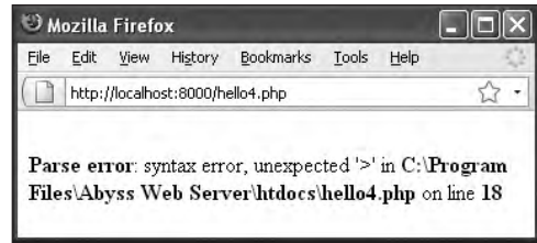
Figure 1.13 Parse errors are frequently caused by an imbalance of quotation marks or parentheses, or by omitting a semicolon.
